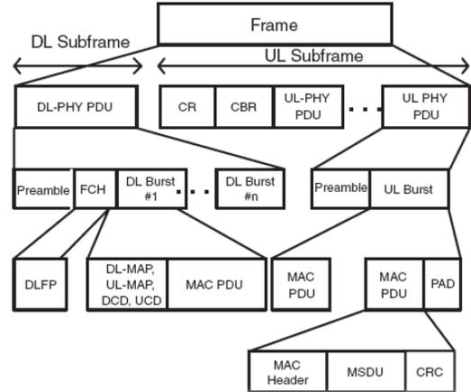
Fig. 1. TDD frame structure for mobile WiMAX [1].
