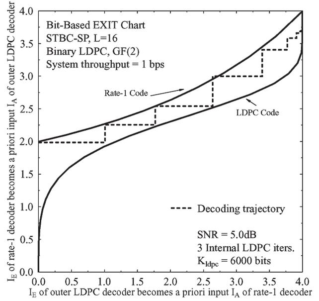
Fig. 5. Decoding trajectory of the bit-based 1/2-rate binary LDPC-coded [5] STBC-SP scheme in combination with the system parameters outlined in Table I and operating at  $E_b/N_0 = 5.0$  dB after 15 joint external iterations and three internal LDPC iterations.
