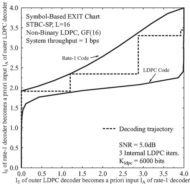
Fig. 4. Decoding trajectory of the symbol-based 1/2-rate nonbinary LDPC-coded [7] STBC-SP scheme defined over  $GF(16)$  in combination with the system parameters outlined in Table I and operating at  $E_b/N_0 = 5.0$  dB after five joint external iterations and three internal LDPC iterations.
