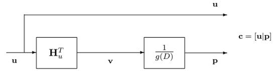
Fig. 3. GeIRA encoder. Decomposing the parity-check matrix as  $\mathbf{H} = [\mathbf{H}_u | \mathbf{H}_p]$ ,  $\mathbf{H}_u$  corresponding to the  $k$  systematic symbols and  $\mathbf{H}_p$  to the  $m = n - k$  parity symbols, we have that  $\mathbf{H}_u^T$  is the outer LDGM code generator matrix. Moreover,  $\mathbf{H}_p$  is specified by the feedback polynomial  $g(D) = \sum_{j=0}^t g_j D^j$  of the inner rate-1 RCC (where  $g_j \in \{0, 1\}$  and  $g_0 = g_t = 1$ ).
