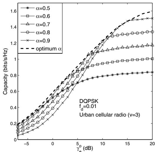
Fig. 2. Capacity of the single-relay-aided DDF cooperative system.
