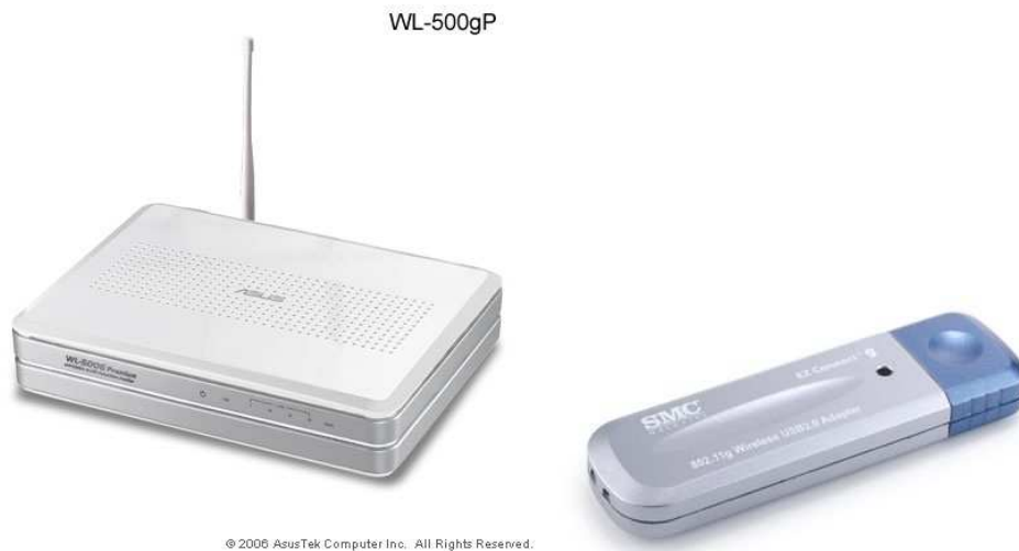
Figure 33 – Access Point and the wireless card.
