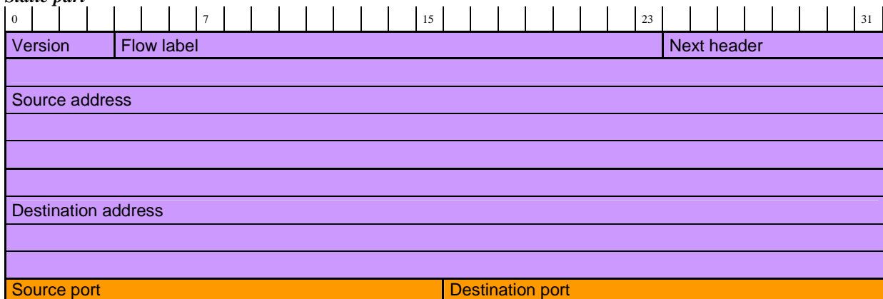
Figure 17 – DCCP/IPv6 static context part (IPv6 fields, DCCP fields).
