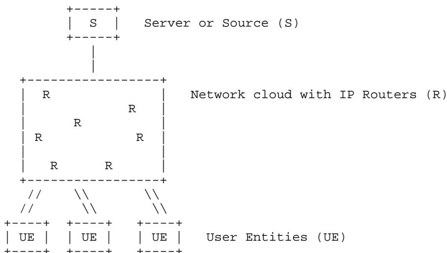
Figure 1 A typical scenario for anycast based aggregation
