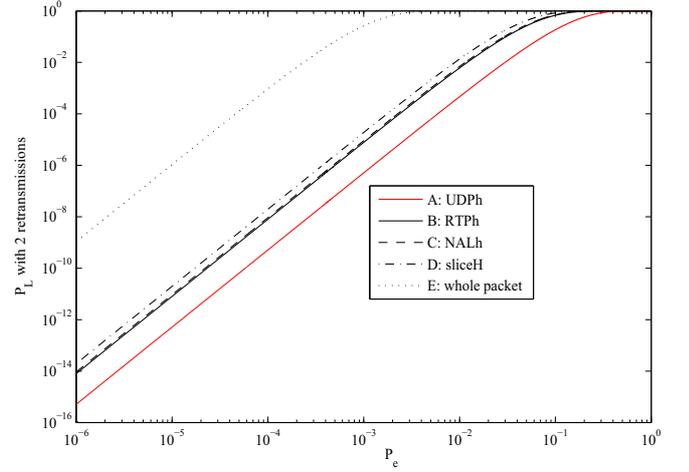
Fig. 4. Packet loss rate vs. bit error probability at the link layer, ARQ with max 2 retransmissions.
