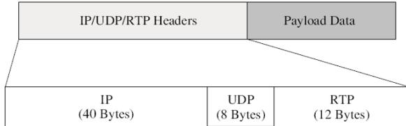
Fig. 1. RTP/UDP/IP packetization.
