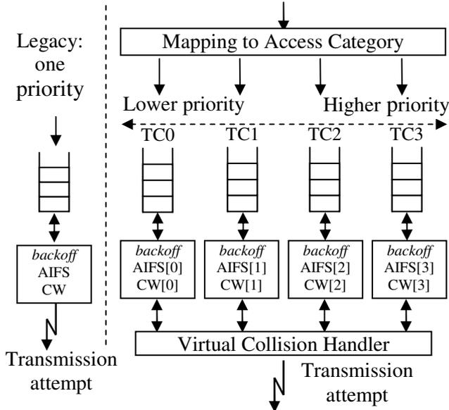
Figure 2: Virtual backoff of Traffic Categories (TCs) with DCF (left) and EDCA (right) methods.
