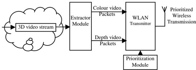
Figure 1: The block diagram of the proposed prioritization scheme
