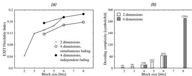
Figure 8: (a) EXIT flexibility index  $F_T$ , when considering different number of bits per joint symbol as well as expanding the modulation constellation from two dimensions to four dimensions for transmission over simultaneous and independent fading based Rayleigh channels. (b) Complexity of schemes in (a).
