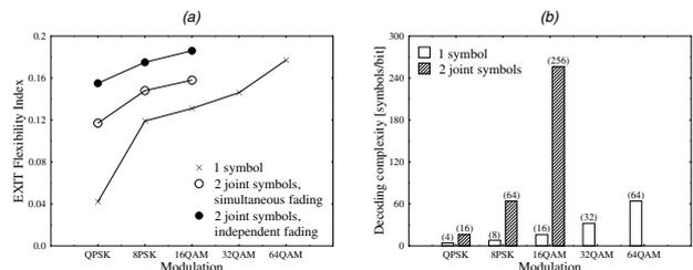
Figure 7: (a) EXIT flexibility index  $F_I$ , when considering different modulation schemes as well as single-symbol decoding and the decoding of two joint symbols, when communicating over simultaneous and independent fading based Rayleigh channels. (b) Complexity of schemes in (a).
