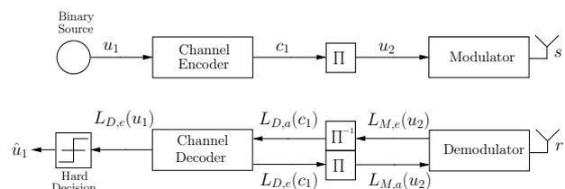
Figure 1: The block diagram of a BICM-ID system.
