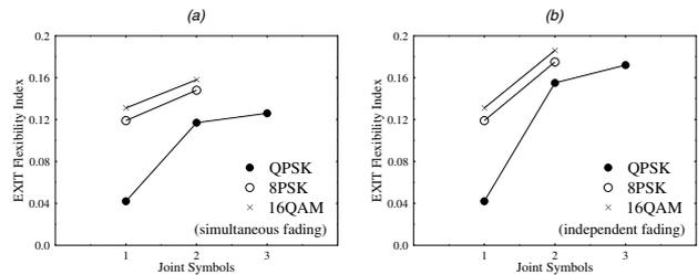
Figure 6: EXIT flexibility index  $F_I$ , when considering various number of joint symbols and different modulation schemes. (a) The case of a simultaneous fading based Rayleigh channel model. (b) The case of an independent fading based Rayleigh channel model.
