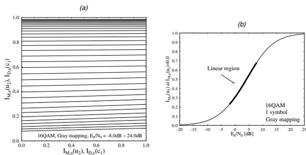
Figure 5: (a) Extrinsic information  $I_{M,e}$  at the output of the demodulator of the BICM-ID scheme of Figure 1, when employing GM-based 16QAM and increasing the SNR in 0.5dB steps from  $E_b/N_0 = -8.0$ dB to  $E_b/N_0 = 24.0$ dB. (b) The improvement of the extrinsic information  $I_{M,e}$  at the output of the demodulator upon increasing the SNR, when no *a priori* information is available at the input of the demodulator.
