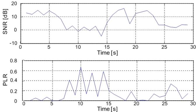
Fig. 5. Detected SNR and PLR of the non-selective block fading channel
