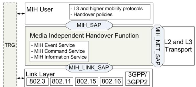
Fig. 2. The General Reference Architecture of IEEE 802.21 Embedded in the Presented Architecture
