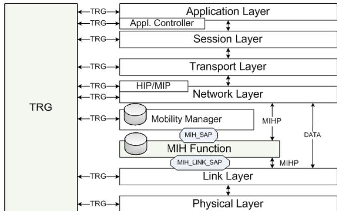
Fig. 6. Schematic of the Internal Architecture of MN
