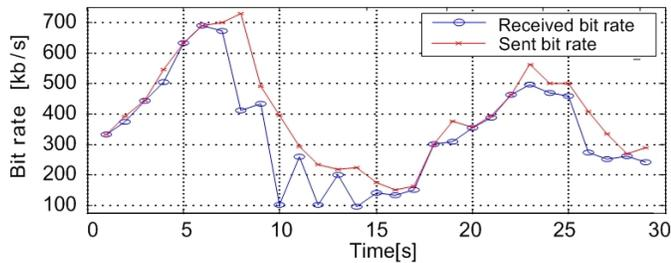
Fig. 4. Adapted bit rate of SVC video stream and an estimate of received bit rate
