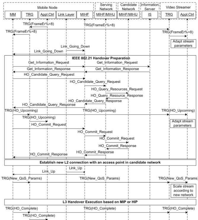
Fig. 7. Sequence Diagram for Simple Use Case Scenario
