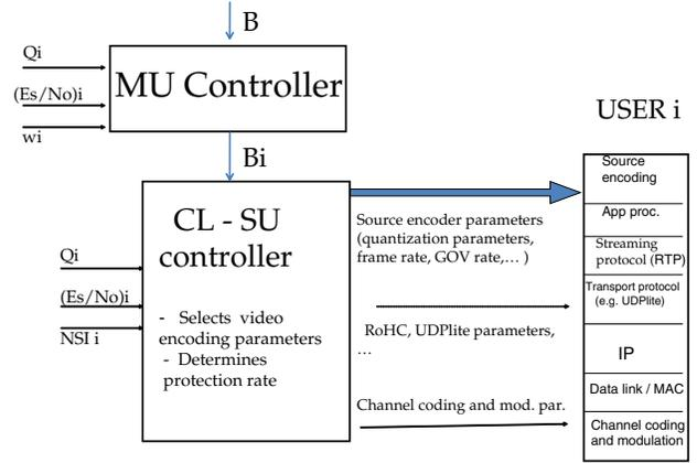
Fig. 2. System controllers
