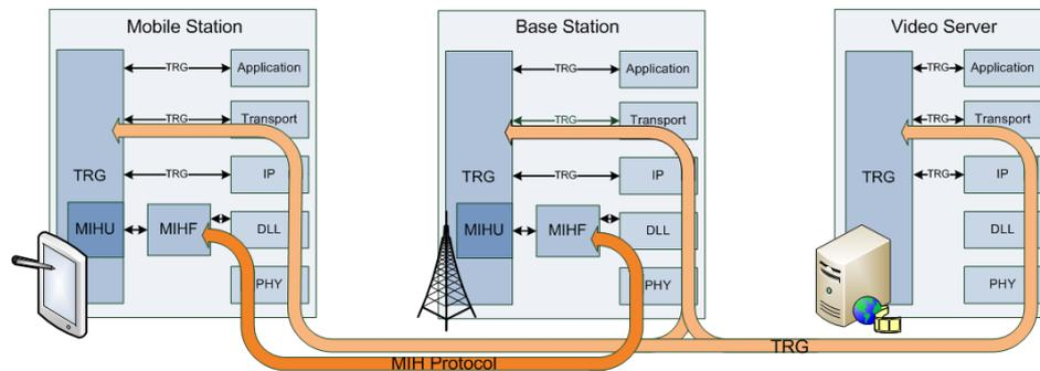
Figure 4: OPTIMIX Cross-layer Signalling Architecture
