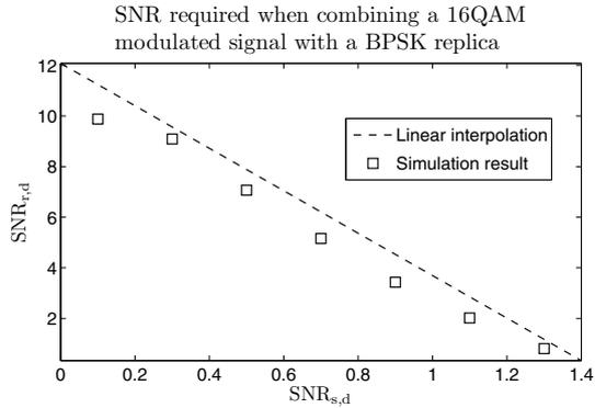
Fig. 1. The SNR required for a 16QAM modulated signal on the RD link when combined with a BPSK signal on the SD link.
