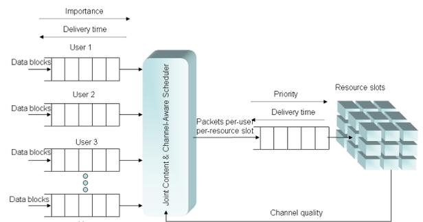
Fig. 1. Schematic of joint content/channel aware scheduling
