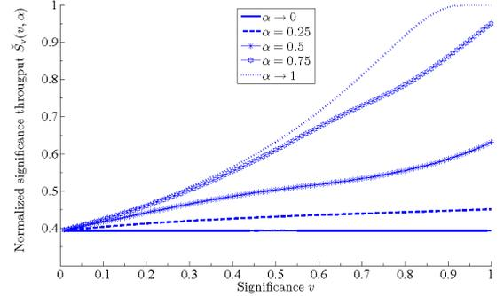
Fig. 5. Normalized significance throughput versus significance for a normalized offered load=1.
