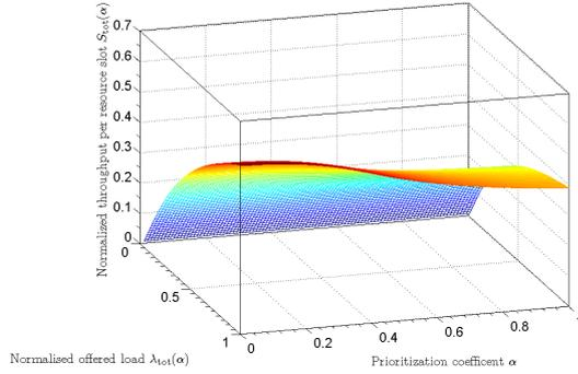
Fig. 2. Normalized throughput per resource slot versus normalized offered load and prioritization coefficient.
