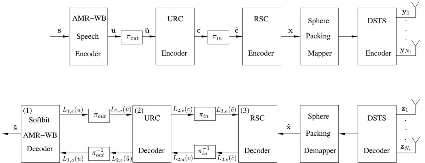
Figure 1: Block diagram of the DSTS-SP-RSC-URC-AMRWB scheme.
