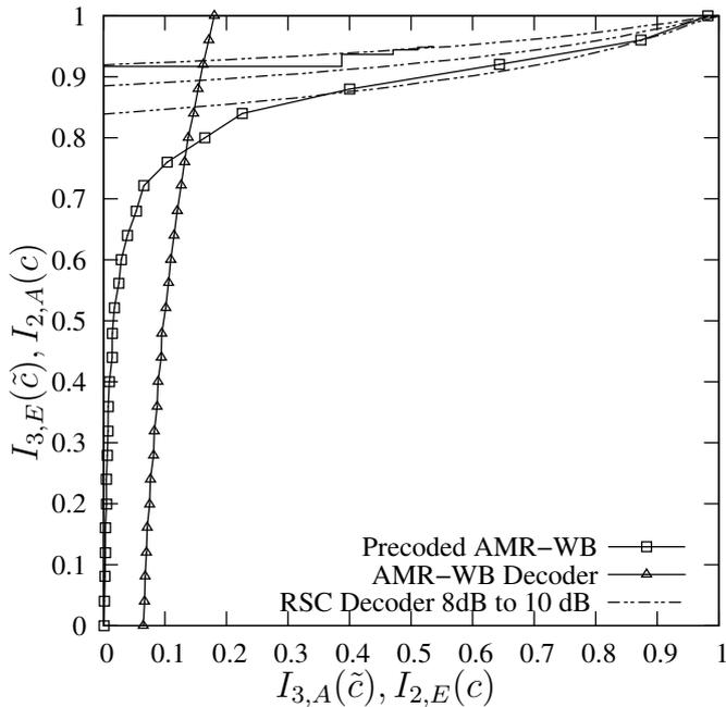
Figure 4: 2D projection of the EXIT chart of the three-stage DSTS-SP-RSC-URC-AMRWB scheme and the 2D EXIT chart of the two-stage DSTS-SP-RSC-AMRWB benchmarker scheme.
