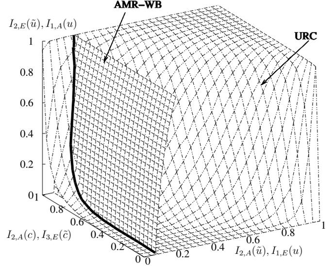
Figure 2: 3D EXIT chart of the URC decoder and of the AMR-WB decoder.
