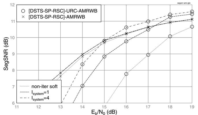
Figure 6: Average SegSNR versus  $E_b/N_0$  performance of the jointly optimised DSTS-SP-RSC-URC-AMRWB scheme of Figure 1 in comparison to the DSTS-SP-RSC-AMRWB benchmark scheme, when communicating over narrowband temporally correlated Rayleigh fading channels.
