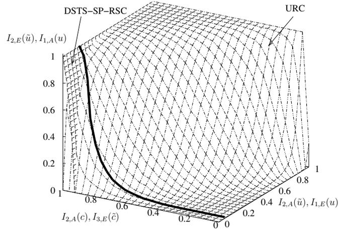
Figure 3: 3D EXIT chart of the URC and the RSC decoders for the two-transmit-antenna aided DSTS-SP system at  $E_b/N_0=10.0$  dB with projection from Figure 2.
