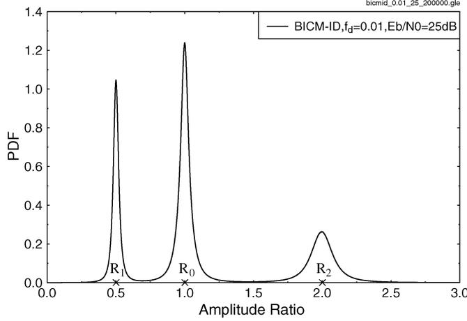
Fig. 2. The PDF of the received signal amplitude ratios of 16StQAM  $|y_k|/|y_{k-1}|$  based on (6), when communicating over correlated Rayleigh fading channels having an  $E_b/N_0$  of 25 dB.
