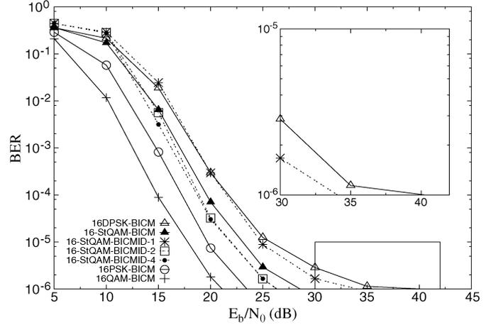
Fig. 3. BER versus  $E_b/N_0$  performance of the 16DPSK-BICM, 16-StQAM-BICM, 16-StQAM-BICM-ID, 16PSK-BICM, and 16QAM-BICM schemes. The simulation parameters are shown in Table I.
