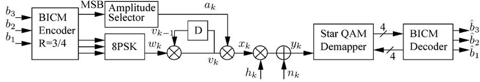
Fig. 1. Schematic of the 16-StQAM aided BICM-ID scheme, where the parallel bit interleavers between the encoder/decoder and mapper/demapper are not shown for avoiding obfuscating details.
