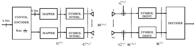
Fig. 2. Architecture of pragmatic space-time codes. In cooperative P-STC, instead of  $n$  we must consider the overall number of antennas  $(R + 1)n$  and the convolutional encoder is the ensemble of single encoders, one for each transmitter (source +  $R$  relays).
